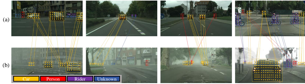
Figure 5: Post-hoc visualization of cross-domain object correspondence from Cityscapes to Foggy Cityscapes. (a) Source domain images (Cityscapes) and (b) target domain images (Foggy Cityscapes). Note: During adaptation, our method never accesses source images; this visualization is created after training solely to illustrate the learned cross-domain semantic alignment.
