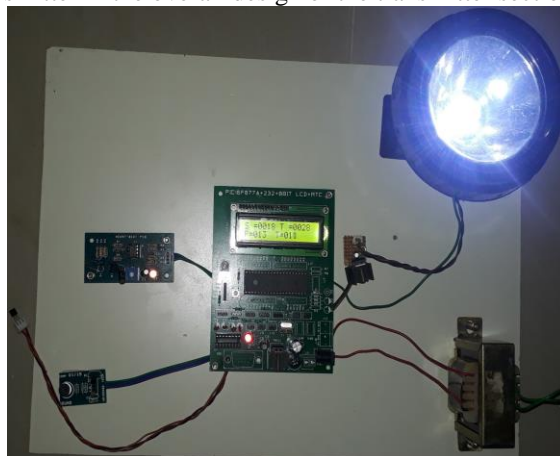
Figure 5. Working model of transmitter for HMS using VLC
