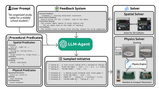
Figure 2: Our framework consists of three components: (a) an LLM agent that takes a user prompt and generates spatial and physical predicates, along with object descriptions for retrieval; (b) a solver that computes the final scene using a physics engine for physical predicates and a sample-based constraint solver for spatial predicates; and (c) a feedback system that reports success or diagnoses failure, allowing the LLM agent to iteratively refine and regenerate predicates.
