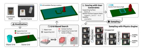
Figure 4: The stacking generation pipeline uses an occupancy-grid-based heuristic to efficiently compute candidate placement locations via grid search, which are then ranked by user requirements. A physics simulator verifies physical validity (e.g., whether an object will fall), and probabilistic programming further assesses stability, enabling control over the robustness of valid states.
