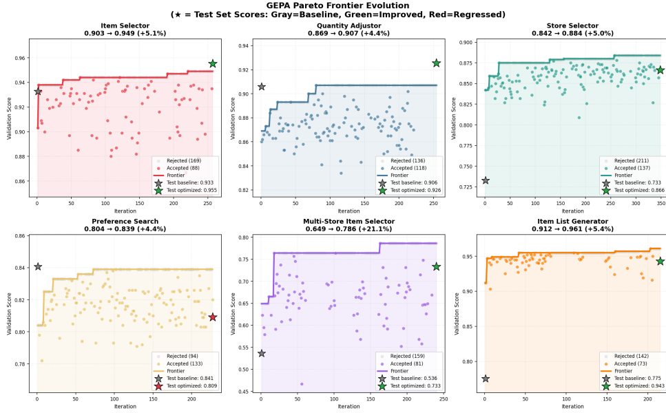
Figure 2: Sub-agent GEPA rubric scores vs. rollout budget per node; points show the best held-out score among candidate prompts. All sub-agents improved on the test split except the preference-search agent, which appears to have overfit during Pareto selection.
