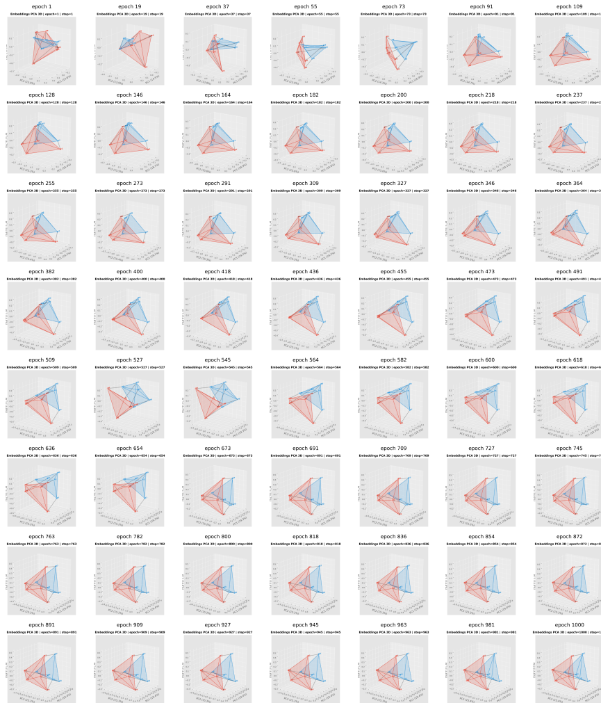
Figure 12: Dynamics of PCA visualizations of entity embeddings throughout training. Each panel shows the projection of embeddings at a different training epoch. In early stages, embeddings are largely unstructured and overlapping. As training progresses, coherent geometric structure gradually emerges, with entities organizing according to their underlying relational roles. This illustrates that structural alignment in representation space is not present initially but forms progressively during optimization.
