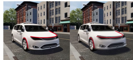
Fig. 4. Left depicts the appearance of a vehicle with its nose down as it is braking. Right depicts the car with its nose raised with an overlay of its previous nose dive state in red.
