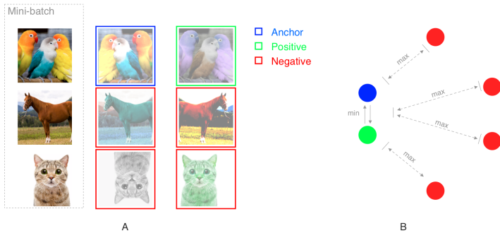
Figure 1: (A) The contrastive self-supervised pretext task consists of finding ways to generate anchor, positive and negative features used as training signals for unlabeled datasets. (B) The positive and anchor pairs are pushed close together, and away from the negative features.
