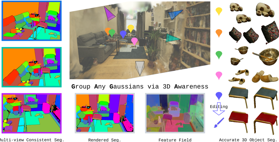
Figure 1: Gaga groups any Gaussians in an open-world 3D scene and renders multi-view consistent segmentation (pixels of the same region across views are represented with the same color). By employing a 3D-aware memory bank, we eliminate the label inconsistency that exists in 2D segmentation predicted by foundational models and assign each mask across different views a universal group ID. This enables the process of lifting 2D segmentation to a consistent 3D segmentation. Gaga produces accurate 3D object segmentation, achieving high-quality results for downstream applications such as scene manipulation (e.g. changing the cushion’s color of the footstool to maroon).
