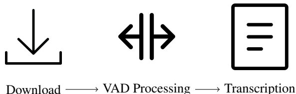
Figure 1: Illustration of the Data Pipeline: (1) Downloading the data in accordance with data creator agreements, (2) Processing Voice Activity Detection (VAD) to segment audio based on silences, and (3) Transcribing the segmented audio, which currently relies solely on machine-based process but is planned to incorporate human transcription.
