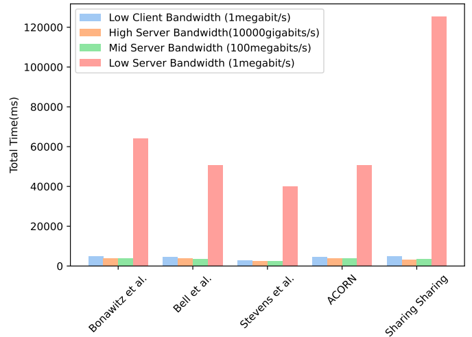
Fig. 9: Effect of bandwidth limitations on total running time (semi-honest security), with 64 clients and length-100 vectors. Limits on client bandwidth have a small impact, but limits on server bandwidth have a large impact.
