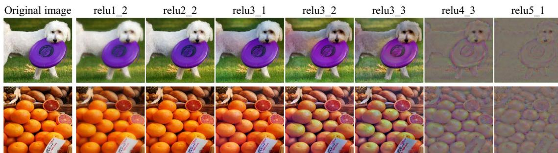
**Fig. 3** Examples of the feature reconstruction for several layers from the VGG-16 pre-trained network
