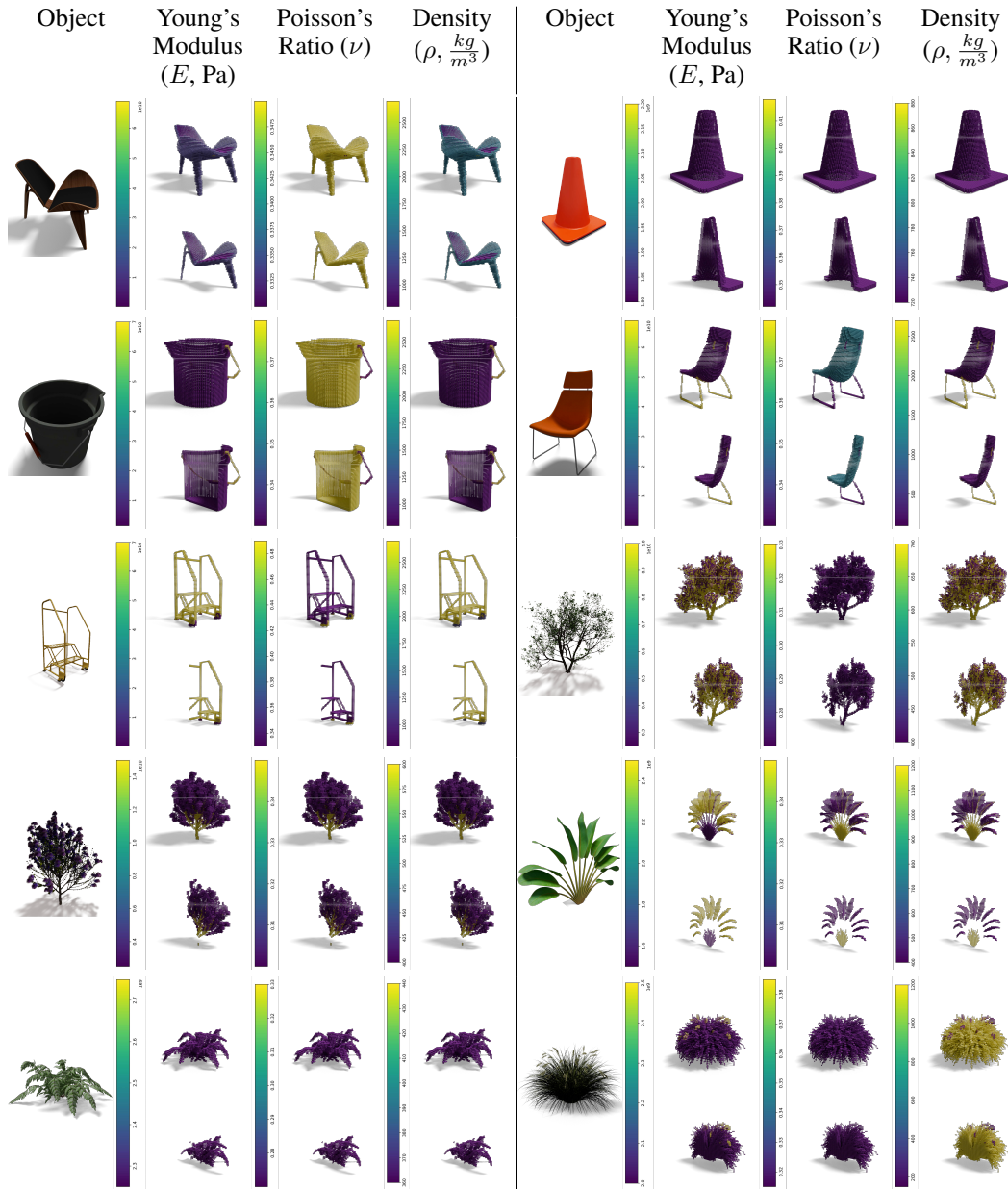
Figure 10: Inferred Mechanical Property Fields. We show additional mechanical property fields and slice planes through mechanical property fields estimated by VoMP (📺 2:10).
