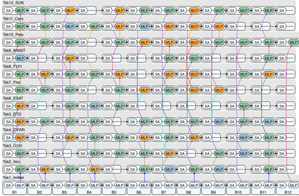
Figure 7: ViT-Base trained on Tsk1_ImNet (with blocks B1 to B12), with Pure Exploration in CHEEM. While pure exploration accounts for task complexity through the skip operation, it also adds more many more Adapt and New operations as compared to the proposed Hierarchical Exploration-Exploitation scheme (Figure 6). This shows that the HEE sampling scheme can effectively leverage task synergies and reuse previous parameter memories.
