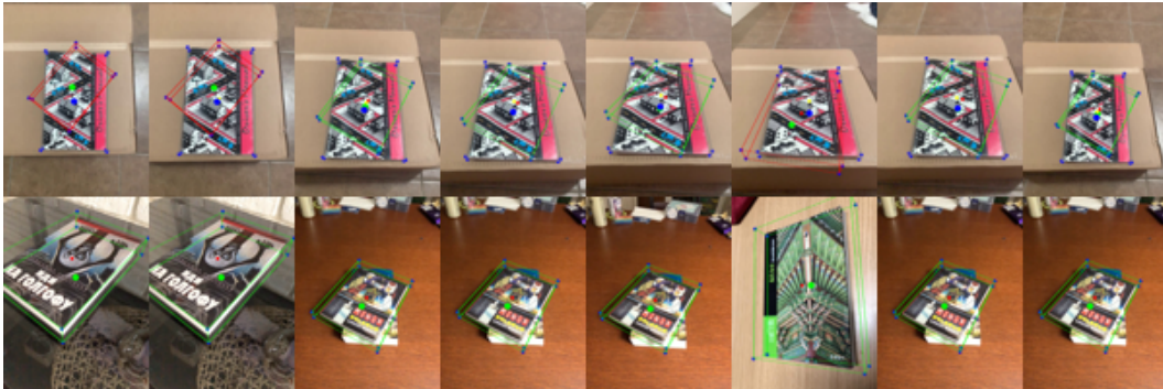
Figure 9: Example of degraded book pose estimation. The orientation of the pattern on the book seems to confuse the pose estimation. Query frames are shown in the top row, nearest neighbors in the bottom row.
