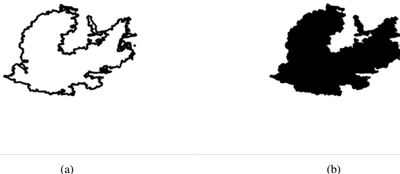
Figure 2: An example of preprocessing wildfire perimeter. (a) A fire perimeter is plotted. (b) Fire perimeter is shaded in to create a binary map.
