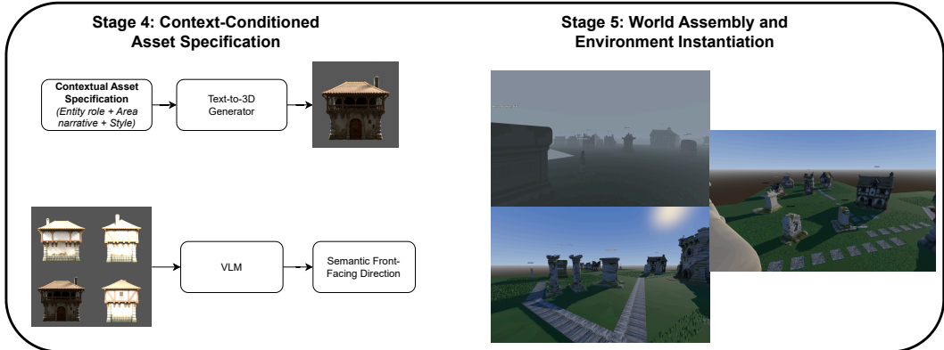
Figure 2: Context-conditioned asset grounding and world assembly. Given the resolved tile-based world layout, context-conditioned 3D assets are generated for each entity by conditioning text-to-3D prompts on the entity’s semantic role, local area narrative, and global style constraints (Stage 4). Because text-to-3D models produce meshes with arbitrary orientation, canonical front, back, left, and right views are rendered and a vision-language model is used to identify the semantic front-facing direction when required. The resolved tile-based layout and oriented assets are then deterministically assembled into an executable environment instantiated in the Godot engine, producing a coherent and traversable 3D world (Stage 5).
