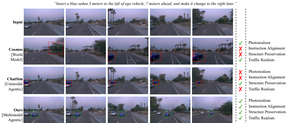
Fig. 1: Natural-language editing. Cosmos [3] achieves high visual quality but fails to align with the target behavior and modifies the background, showing poor controllability. While ChatSim [41] preserves background information, it suffers from poor photorealism, inaccurate trajectory generation, and traffic violation (e.g., collision). In contrast, our method achieves photorealism, instruction alignment, structure preservation, and traffic realism simultaneously, significantly outperforming previous methods.
