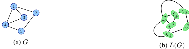
Figure 2: An example of a graph and the corresponding line graph. The edges in G are the nodes in L(G) , and vice-versa.
