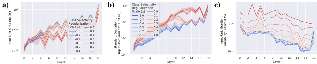
Figure A19: Mean and standard deviation of input-unit gradient in ResNet20 trained on CIFAR10. (a) Input-unit gradient (y-axis) as a function of layer (x-axis). (b) Standard deviation of input-unit gradient for each unit ( \sigma_u ; y-axis) as a function of layer (x-axis). (c) Standard deviation of input-unit gradient across units in a layer ( \sigma_l ; y-axis) as a function of layer (x-axis). Shaded region = 95% confidence interval of the mean.
