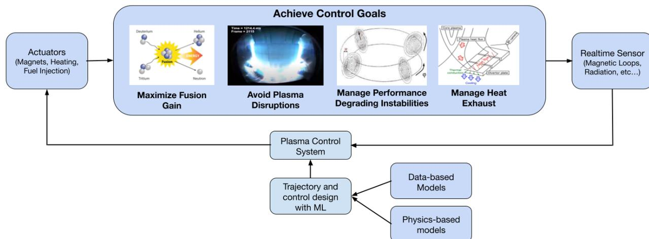
Figure 3. Diagram showing important goals for advanced control research to address along with key relevant components. Inspiration for the diagram was taken from (Humphreys et al., 2019). Credit for embedded figures, from left to right: (Gunn, 2022), (IPP, 2017), (Igochine), (Hayashi et al., 2021).
