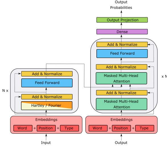
Figure 2: Right-side Attention Encoder-Decoder (RAED) diagram. We tested also another configuration where we replaced these two Multi-head Attention green boxes with a Hartley/Fourier in the same manner as was done by Kiruluta et al. (2021), the so-called FNet-Transformer, but without equal success as RAED with downstream tasks.
