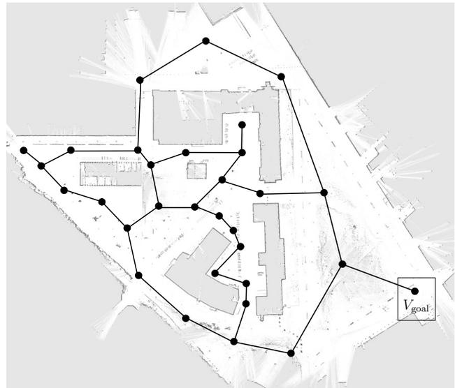
**Figure 1.** Initial working example: A mobile robot navigates in a planar environment amongst obstacles. For simplicity, a generalized Voronoi graph is superimposed over the top; the robot can start anywhere and we desire that it navigate toward the region represented by the rightmost vertex. (This is part of the University of Freiburg campus, with thanks to Cyrill Stachniss and Giorgio Grisetti for making the dataset available.)
