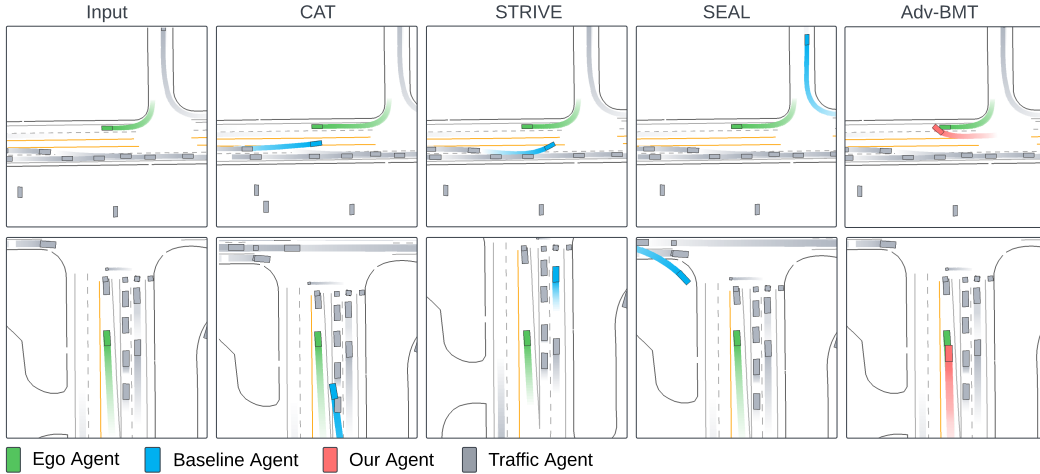
Figure 7: Baseline method comparisons. We present several examples where Adv-BMT successfully generates collision interactions in scenarios where all baseline methods fail. Unlike the baselines, Adv-BMT does not rely on the proximity of neighboring agents to the ego vehicle, enabling more flexible and diverse adversarial attack strategies.
