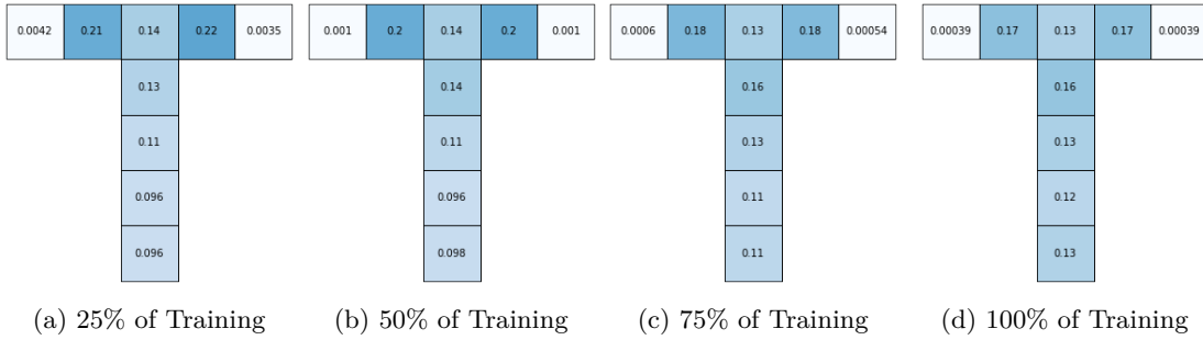
Figure 3: TMaze Fixed Model Solution: the evolution of MGSC’s learned search control distribution during the fixed model experiment. Each figure shows MGSC’s learned search control distribution, represented by the parameter vector \eta , at a different point during training. The number overlaying each state represents the probability that the corresponding state of MGSC’s TMaze model will be sampled during a planning step. Darker colors indicate greater probability mass. The distribution is initialized uniformly, but as shown in the Figure, by 25% of training, MGSC’s meta-gradient updates have shifted probability away from the states adjacent to terminal states. As the model’s terminal states produce erroneous rewards, MGSC learns to avoid planning using them.
