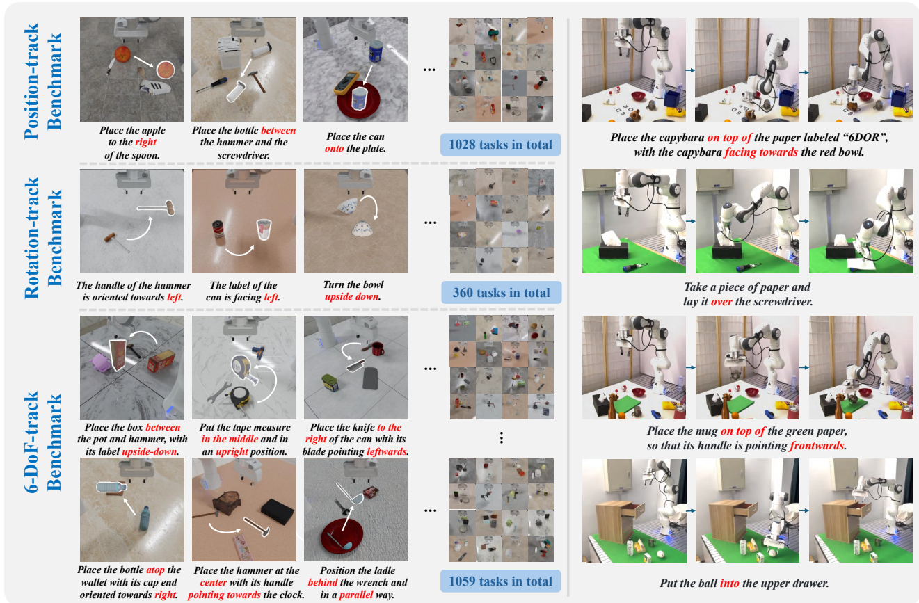
Fig. 1: Open6DOR Benchmark and Real-world Experiments. We introduce a challenging and comprehensive benchmark for Open-instruction 6-DoF object rearrangement tasks, termed Open6DOR. Following this, we propose a zero-shot and robust method, Open6DOR-GPT, which proves effective in demanding simulation environments and real-world scenarios.
