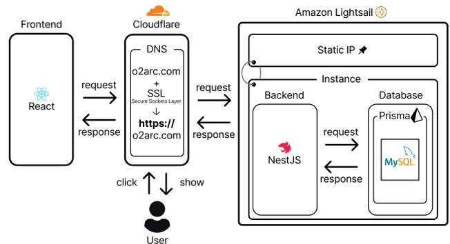
Figure 3: System design of the O2ARC 3.0.
