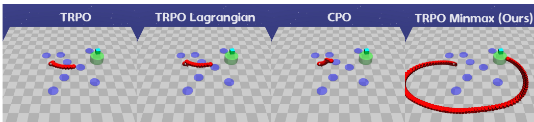
Figure 1: Sample trajectories of representative prior works—TRPO (Schulman et al., 2015) (left-most), TRPO-Lagrangian (Ray et al., 2019) (middle-left), CPO (Achiam et al., 2017) (middle-right)—compared to ours (right-most) in the Safety Gym domain (Ray et al., 2019). For each, a point mass agent learns to reach a goal location (green cylinder) while avoiding unsafe regions (blue circles). The cyan block is a randomly placed movable obstacle. Our approach learns safer policies than the baselines, and works by simply changing the rewards received for entering unsafe regions to a learned penalty (keeping the rewards received for all other transitions unchanged).
