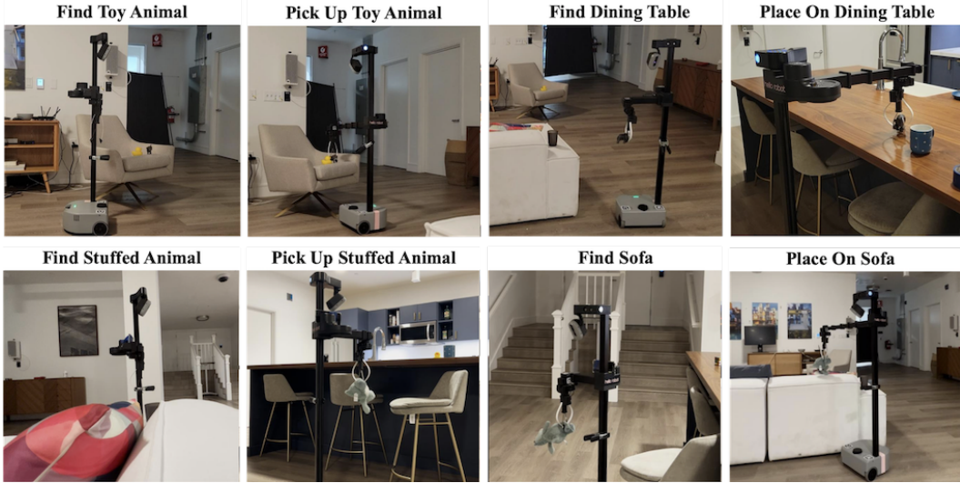
Figure 17: Real-world examples (also see Fig 2). Our system is able to find held-out objects in an unseen environment and navigate to receptacles in order to place them, all with no information about the world at all, other than the relevant classes. However, we see this performance is highly dependent on perception performance for now; many real-world examples also fail due to near-miss collisions.
