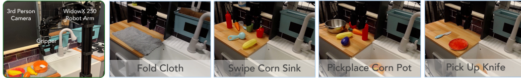
Figure 5: Real robot setup. We design 4 real-world robot tasks with different manipulation skills and objects.
