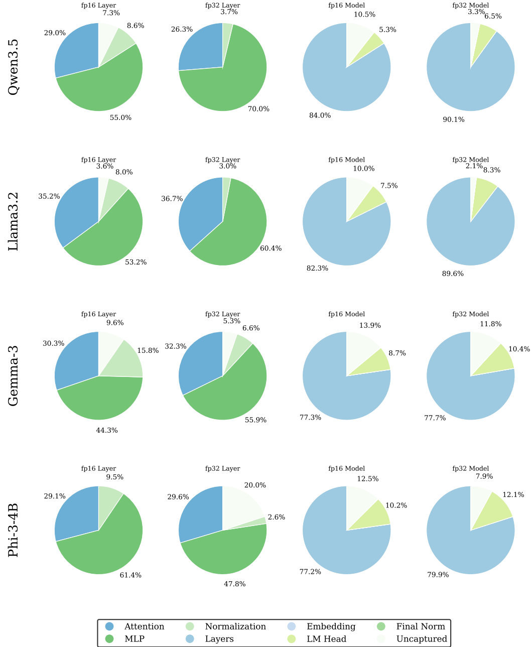
Figure 9: Energy breakdown in decoder-only models. The first two charts illustrate block-level distributions, while the latter two present distributions across the entire model. FP-16 and FP-32 precisions for each model are shown.
