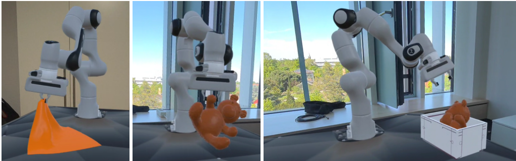
Figure 18: Views wearing a VR headset and collecting task demonstrations using IRIS with IsaacLab. Tasks from left to right are: folding a cloth in half, lifting a deformable teddy, and stowing a deformable teddy in a slightly undersized box.
