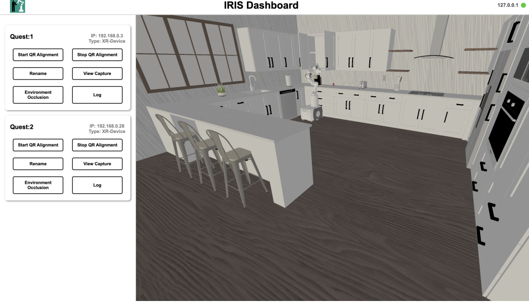
Figure 15: The IRIS Dashboard, accessible via a web interface, allows the control and monitoring of all connected nodes. The scene streamed by IRIS is rendered on the right-hand side. The left panel displays the connected XR devices, providing an interface through which users can control all services made available by each device.
