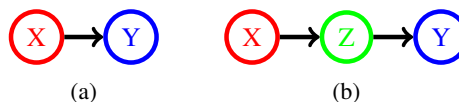
Figure 2: Causal diagram for the medical image segmentation problem. (left) 2a, the standard causal prediction model used for segmentation tasks. (right) 2b, a new mediator variable Z , aimed at addressing data scarcity challenges.
