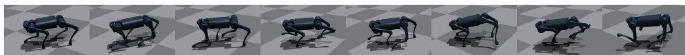
Figure 4: Transition from the 'pace' gait (frame 12) to the 'trot' gait (frame 345), and eventually to the 'gallop' gait (frame 678).
