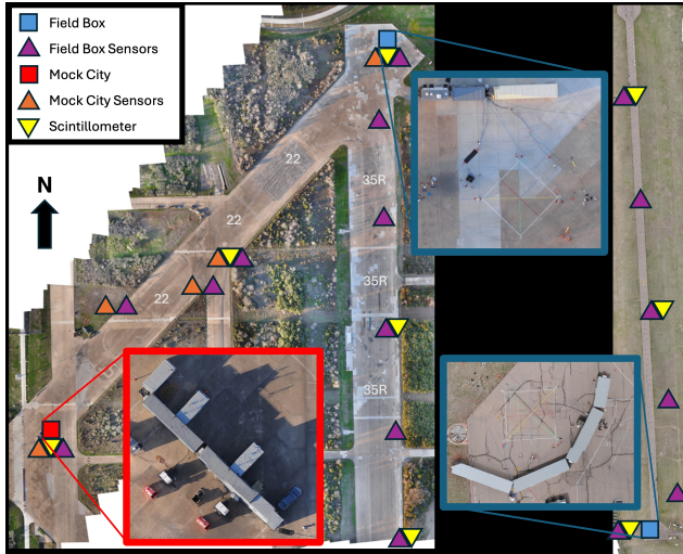
Figure 3. Layout of BGC5 (left) and BGC6 (right). Triangles mark the locations of the camera stations, as well as the scintillometers used to estimate C_n^2 , a measure of atmospheric turbulence. The blue-bordered cutouts show the orientation of the field box for each collection, and the red-bordered cutout shows the mock-city layout.
