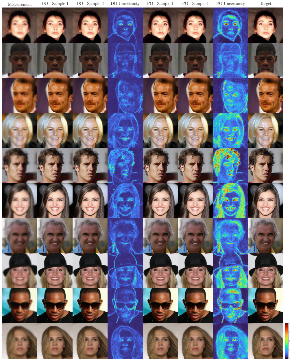
Figure 11: Distortion and Perception optimized deblurring results for the CelebA-HQ dataset (test split). Uncertainty is calculated over n = 10 reconstructions from the same measurement.
