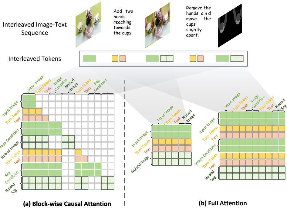
Figure 11: Implementation of (a) block-wise causal attention and (b) full attention.
