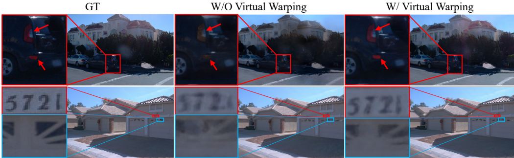
Figure 8: Our virtual warping contributes to color correction (top) and edge sharpness (bottom).
