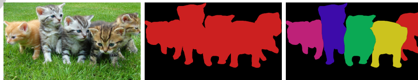
Fig. 2. Visual representation of the different variants of the image segmentation problem. From left to right, original image, semantic segmentation and instance segmentation examples.
