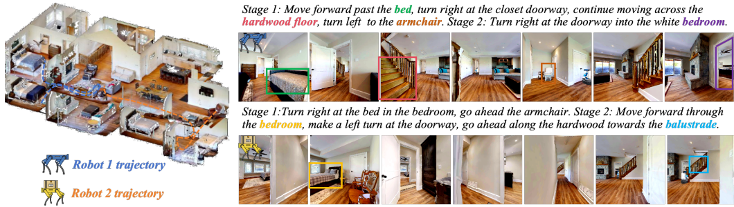
Figure 10: Visualization of cooperative navigation in CoNavBench. Robot 1 and Robot 2 traverse a residential environment along the floor-plan map (left). Colored bounding boxes mark salient landmarks; the same colors are used in the instruction text to denote aligned references. The partner robot can help retrieve visual evidence and disambiguate targets, yielding more efficient progress.
