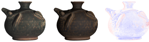
Figure 3: The image of the colored object (left) is very similar to the simulated image (middle). The colors are different due to the lack of calibration during 3D printing. We show the normalized pixel-wise differences in luminance on the right, with the same color scale as used in Figure 1.
