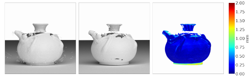
Figure 4: Point clouds from real and simulated scans and their error. The mean error measured with one-sided point-to-point distance is 0.17 mm. Note that some parts of the reconstructed object differ due to lighter and less saturated colors of the 3D-printed object.
