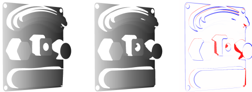
Figure 5: Color-coded (gray-scale) horizontal correspondence indices retrieved from the physical setup (left) and the simulation (middle) for Gray code scanning. The difference between the indices, linearly scaled between -1400 (blue) and 1400 (red) shows large errors only in boundary regions. The average index error is 0.97 (without boundary), and 12.3 (with boundary errors).
