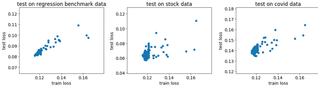
Figure 6: Comparison of loss values between synthetic data and other datasets, where each point corresponds to a hyper-parameter candidate which is obtained during hyper-parameter search. The x -axis and y -axis show loss values on synthetic dataset and other datasets, respectively. The performance on simple synthetic data is highly correlated with the performance on real data.
