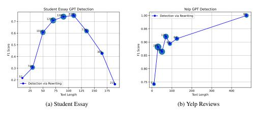
Figure 8: Detection performance under different length. For both datasets, longer length helps detection. Yet, on student essay, input longer than 125 words will lead to performance degradation.
