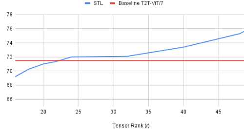
Figure 3: Accuracy \uparrow vs. tensor rank ( r ) for baseline T2T-ViT/7 and for the same architecture with all activation-weight MATMULs in the network trunk replaced by STL with tensor rank r . Very similar picture when including the pre-trunk (T2T) network as a followup experiment.
