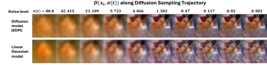
Figure 1: Comparison of Sampling Trajectories. For high to moderate noise levels ( \sigma(t) \in (4, 80] ), the linear denoisers well approximate the learned deep denoisers. Though the two models diverge in lower noise regimes, their final samples still match in overall structure.
