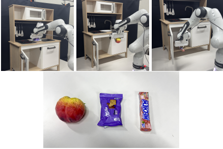
Figure 4: Real-world tasks. We conduct pick-and-place tasks from the countertop to the bottom cabinet with peach, milka, and hichew.
