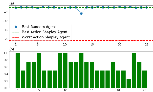
Figure 3: Validation of Action Shapley based selection policy for database tuning. (a) Comparisons of cumulative rewards among the best Action Shapley agent, the worst Action Shapley agent, and the best of 4 random training action sets for 25 different episodes. (b) Fractions of agents based on 4 random training datasets with lower cumulative rewards than that of the best Action Shapley agent for 25 episodes.
