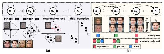
Figure 1: (a) Illustration of attribute loss as time-step t increases in the forward diffusion process. The two axes depict a two-dimensional sample space. (b) DM reconstructed  $\mathbf{x}_0$ , denoted as  $\hat{\mathbf{x}}_0$ , from randomly sampled  $\mathbf{x}_t$  at various t. DM is pre-trained on CelebA, from where  $\mathbf{x}_0$  is drawn.
