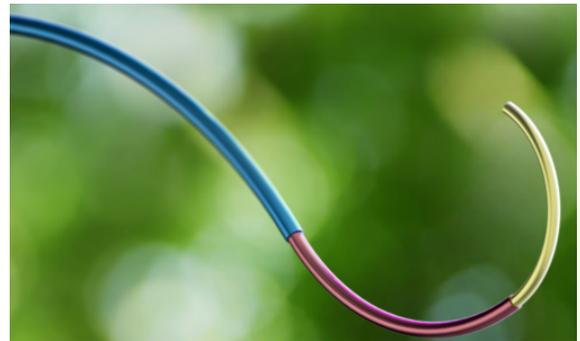
Fig. 1: Rendering of a CTCR (Image from [8]). A CTCR consists of several super-elastic tubes. These are the one of the smallest robot among all continuum robots [16, 35]. According to Burgner-Kahrs et al. [5], these have an ideal structure for the usage in robot-assisted minimally invasive surgery.
