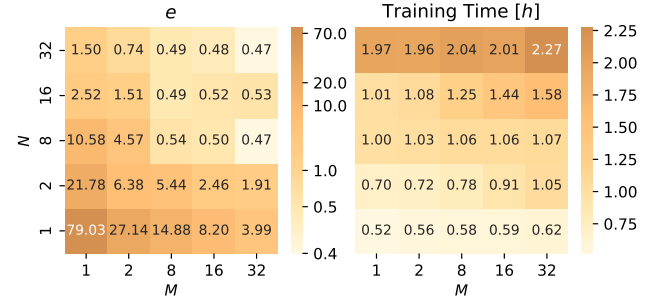
Figure S8. Ablation study on the history horizon M and forecast horizon N in RWM. The heatmap on the left shows the relative autoregressive prediction error, with darker colors indicating higher errors. Models trained with larger history horizons M exhibit lower errors, although the improvements plateau beyond a certain point. Forecast horizon N has a significant impact, with longer horizons leading to better long-term prediction accuracy due to exposure to extended rollouts during training. The heatmap on the right illustrates training time, with darker colors representing longer durations. Increasing N significantly raises training time due to sequential computation, while shorter horizons (e.g., N = 1 , teacher-forcing) enable faster training but result in poor prediction accuracy.
