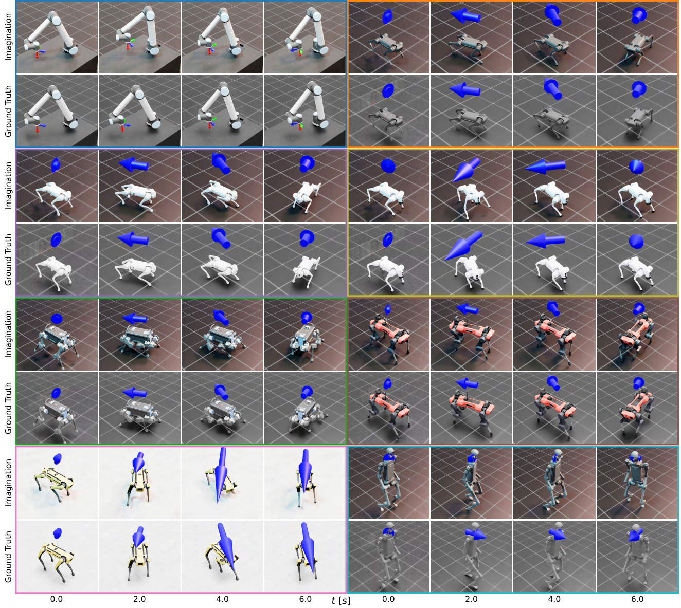
Figure S9. Autoregressive imagination of RWM and ground-truth simulation across diverse robotic systems. For each environment, the top row showcases the RWM autoregressively predicting future trajectories in imagination. The second row visualizes the ground truth evolution in simulation. The visualized coordinate and arrow markers denote the predicted and measured end-effector pose and base velocity, respectively.
