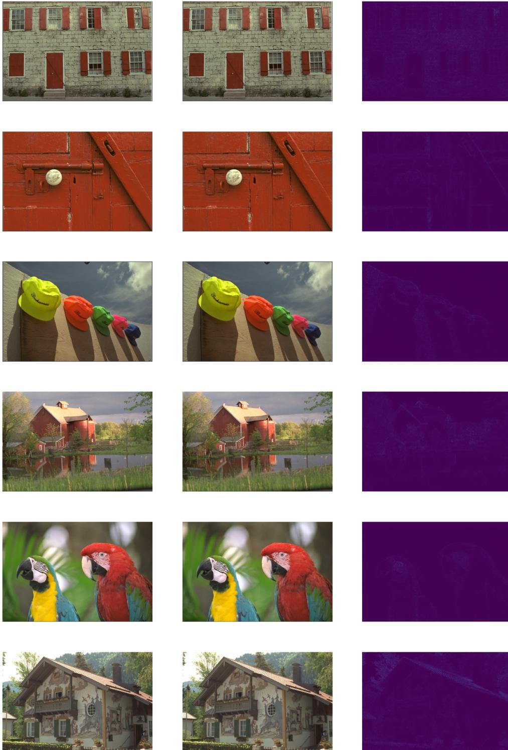
Figure 7. Qualitative results for AE-SIREN on Kodak images. From left to right: original images, decompressed images, and residuals. The model used has the average PSNR of 33.92 and 1.50 bpp.
