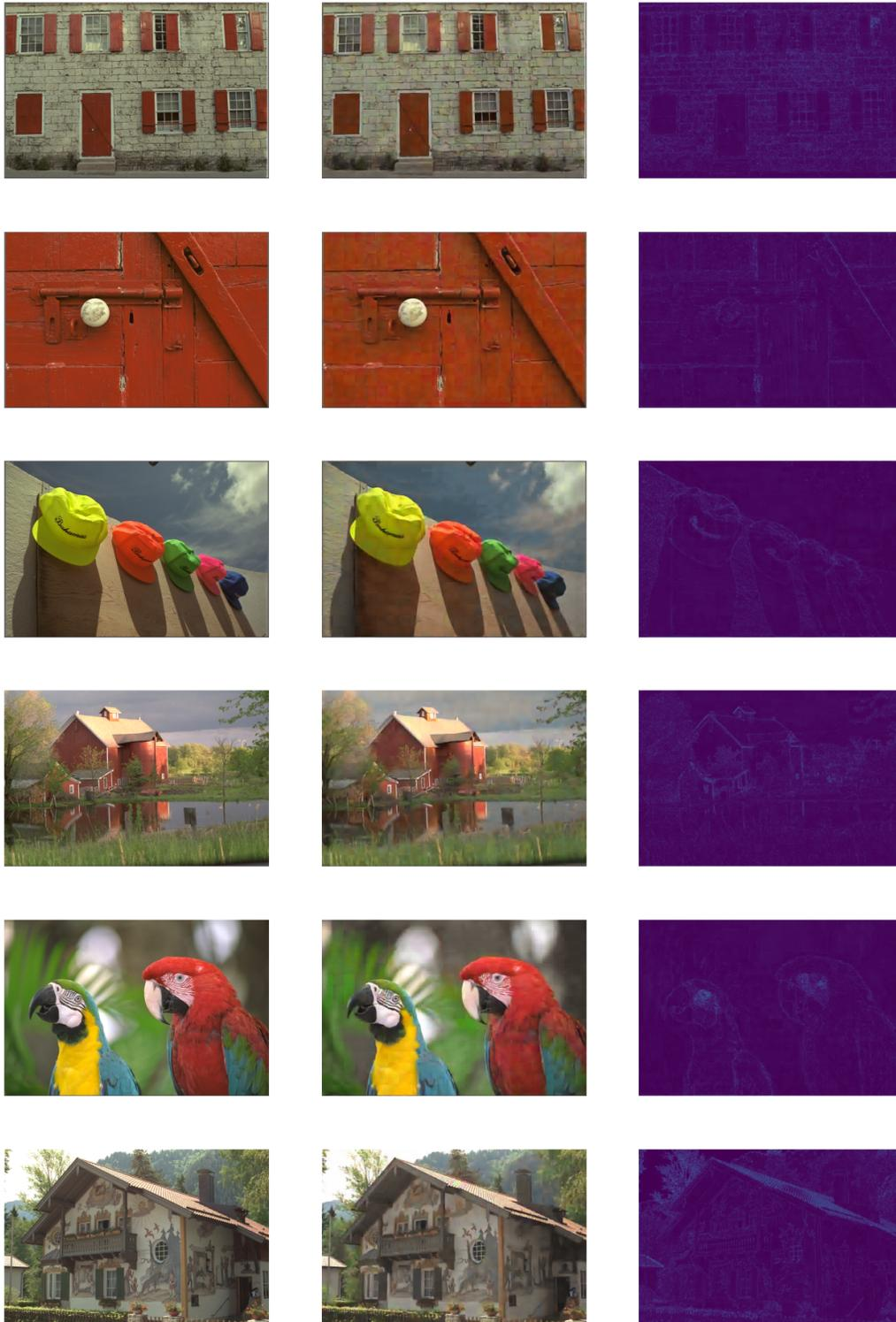
Figure 10. Qualitative results for AE-LIIF on Kodak images. From left to right: original images, decompressed images, and residuals. The model used has the average PSNR of 26.13 and 0.21 bpp.
