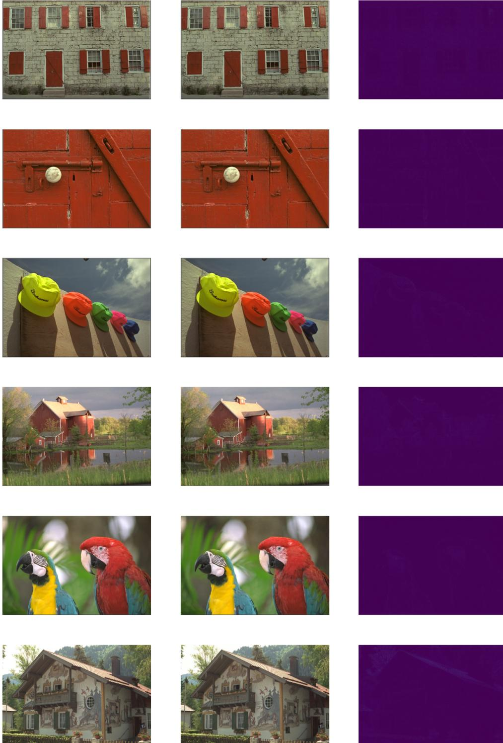
Figure 9. Qualitative results for AE-LIIF on Kodak images. From left to right: original images, decompressed images, and residuals. The model used has the average PSNR of 38.04 and 2.26 bpp.
